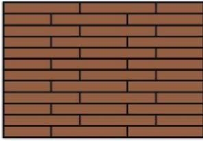
**Less than 16m<sup>2</sup>: full loose lay installation – no expansion gap**
